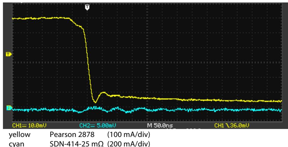
Figure 4.5.2 Responses for Pearson 2878 and 25 mΩ shunt connected with one lead only.
