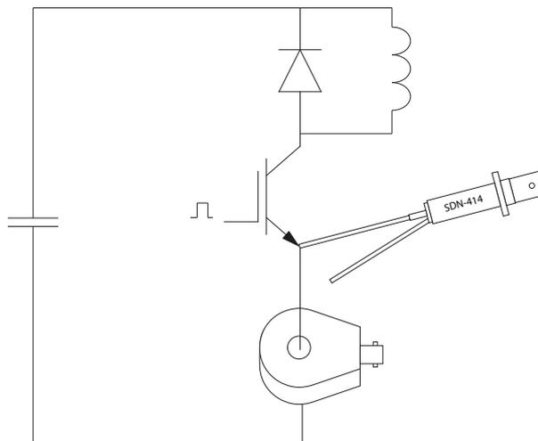
Figure 4.5.1 Test setup for measuring disturbance with shunt only connected with one lead to the circuit.
