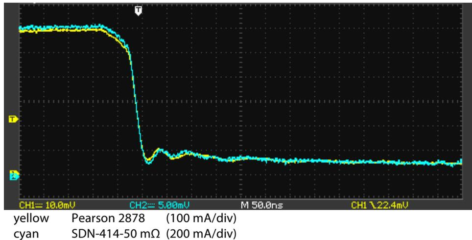
Figure 4.5.3 Responses for Pearson 2878 and 50 mΩ shunt close to an air coil carrying load current.
