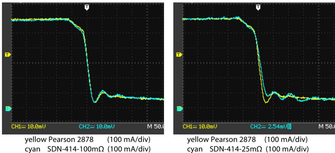
Figure 4.4.2 Responses for Pearson 2878 and 100 mΩ shunt (left) and 25 mΩ shunt (right)
