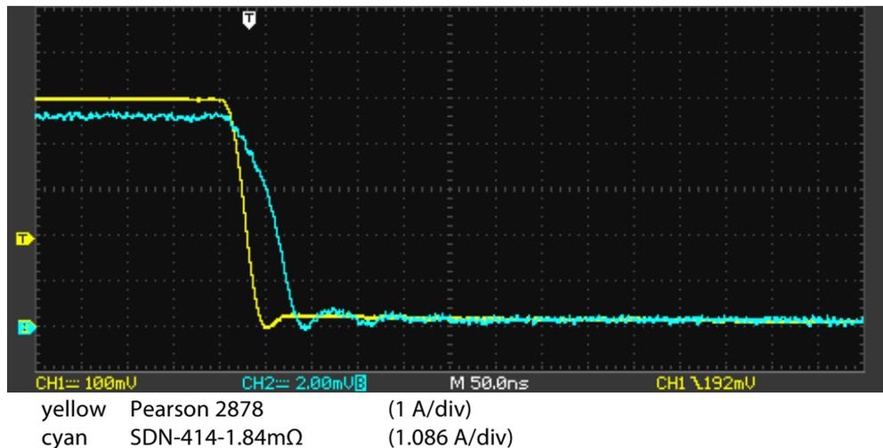
Figure 5.2.3 Responses of Pearson 2878 and the low resistance 1.84mΩ shunt at 5 A in the EMI improved setup.
