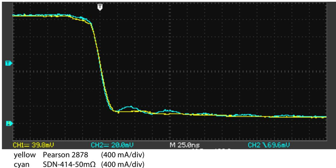
Figure 3.1 Initial result of current waveforms for Pearson 2878 and 50 mΩ shunt.
