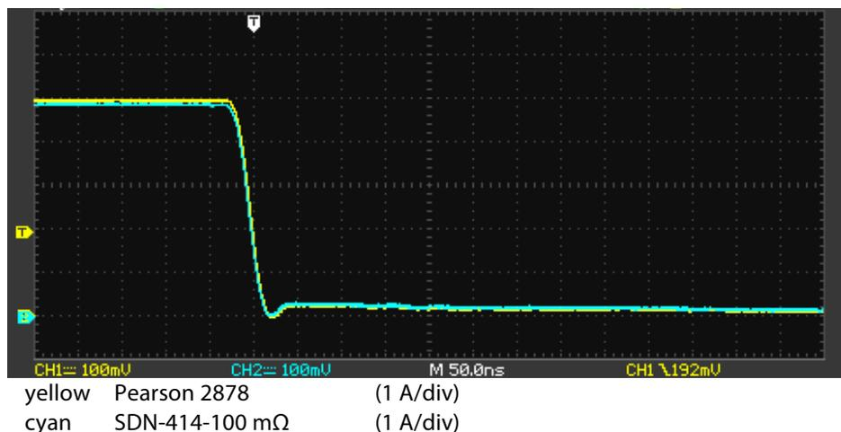
Figure 5.2.2 Responses of Pearson 2878 and 100 m $\Omega$  shunt at 5 A in the EMI improved setup.
