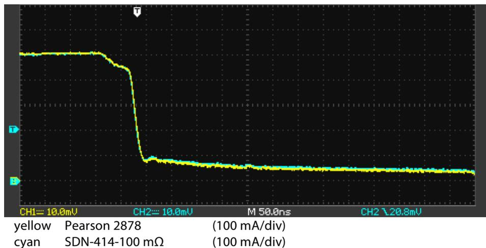
Figure 5.2.1 Responses of Pearson 2878 and 100 m $\Omega$  shunt at 500 mA in the EMI improved setup.
