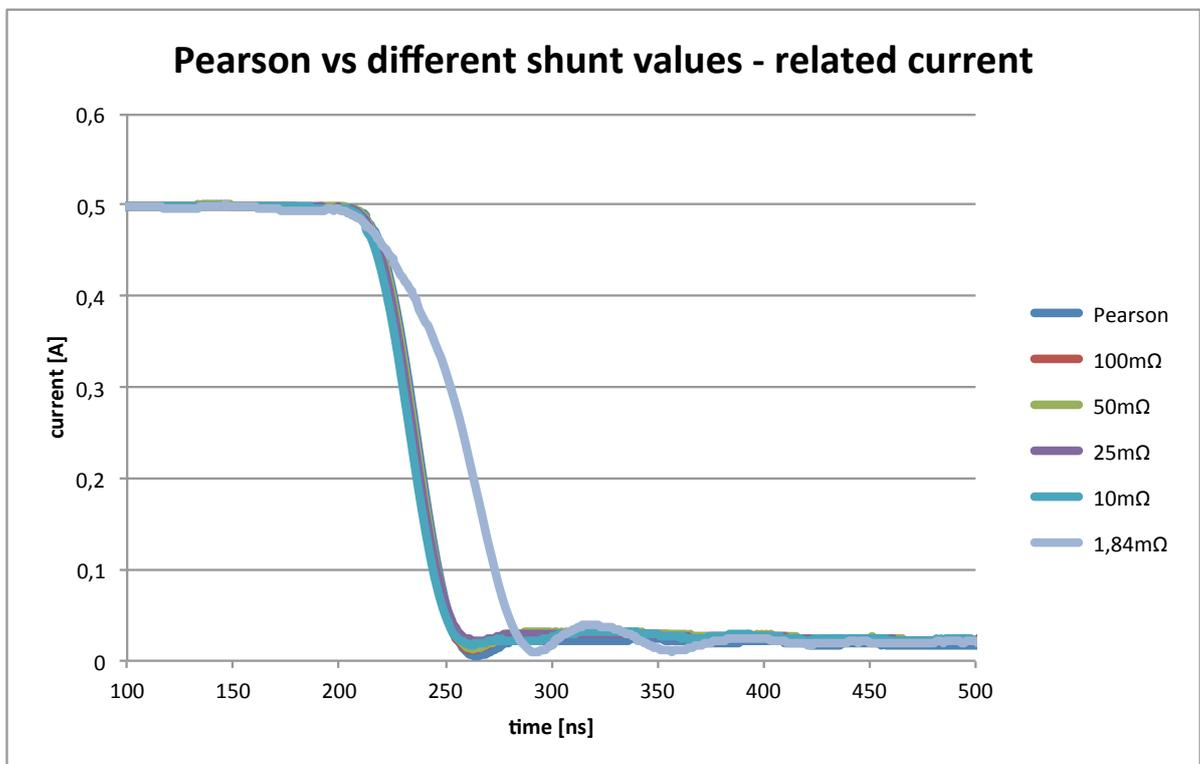
Figure 5.2.7 Measured current by Pearson 2878 different SDN-414 shunts at 5 A.
