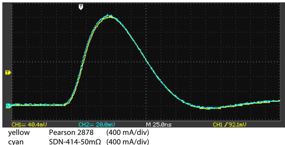
Figure 4.1.3 Identical responses for Pearson 2878 and shunt SDN-414-50 for output current of IGBT gate driver.
