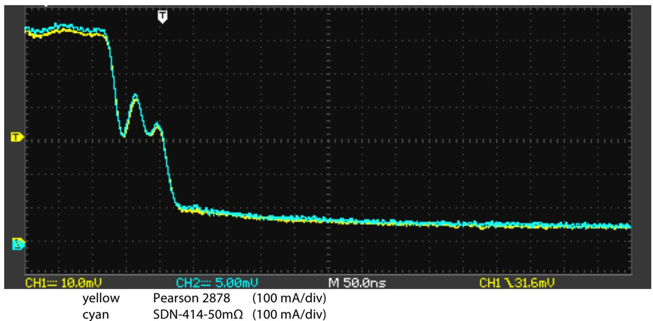
Figure 4.3.1 Identical responses for Pearson 2878 and shunt SDN-414-50 for high frequency oscillation during the slope.
