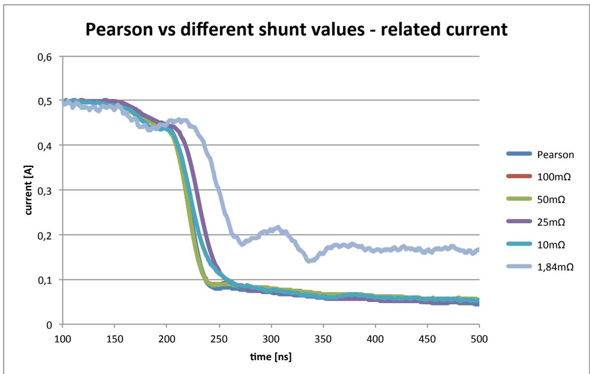
Figure 5.2.5 Measured current by Pearson 2878 different SDN-414 shunts at 0.5 A.
