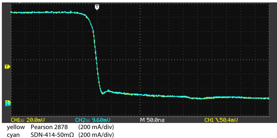
Figure 4.2.1. Identical response for Pearson 2878 and shunt SDN-414-50 for switching a resistive load.
