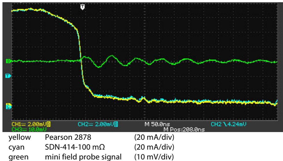
Figure 4.5.7 Responses of 50 mΩ shunt and response of E-probe near core of load coil.
