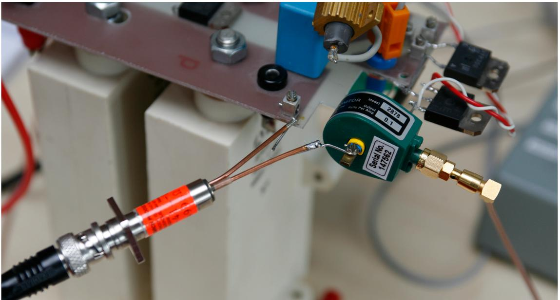
Figure 2.2 Measurement setup for testing Pearson 2878 and 50 mΩ shunt at low currents.
