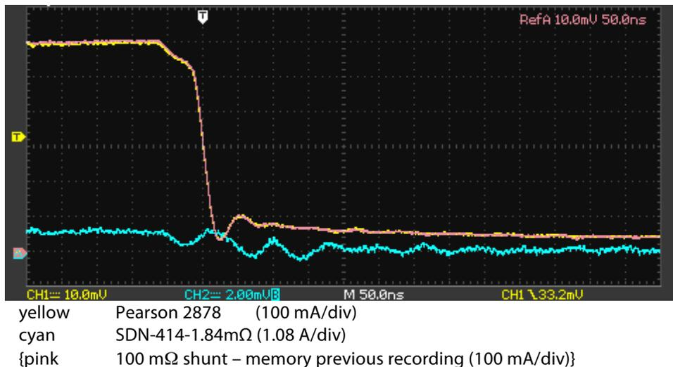
Figure 4.4.3 Responses for Pearson 2878 and 1.84 mΩ shunt at 0.6 A.
