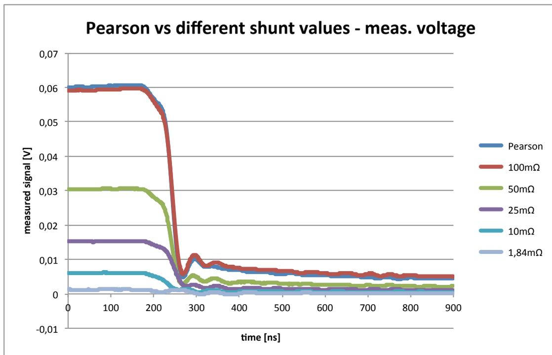
Figure 4.4.4 Recorded voltage by oscilloscope for Pearson 2878 different SDN-414 shunts at 0.6 A.
