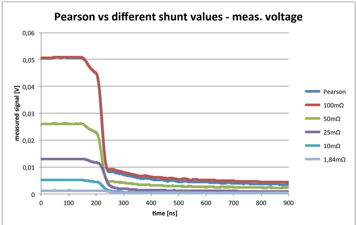
Figure 5.2.4 Recorded voltage by oscilloscope for Pearson 2878 different SDN-414 shunts at 0.5 A.
