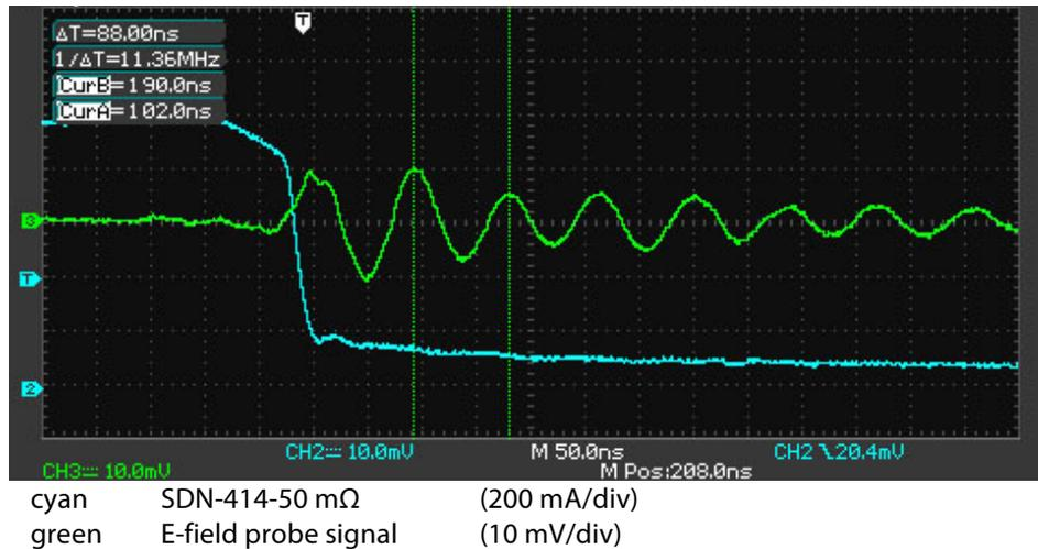
Figure 4.5.6 Responses of 50 mΩ shunt and response of E-probe near leads from DC-bus capacitor to power supply.
