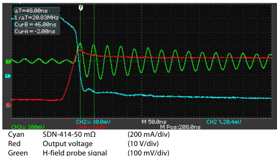
Figure 4.5.4 Responses for 50 mΩ shunt, output voltage and H-field probe close to commutation cell.
