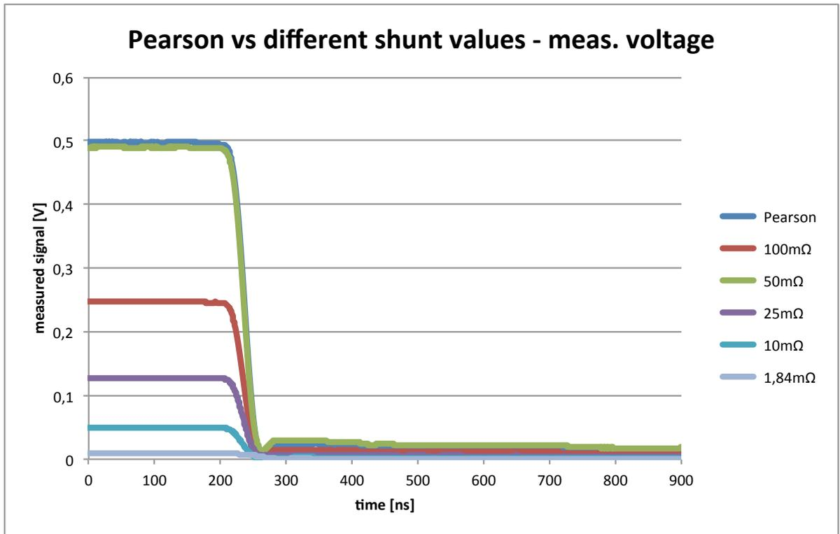
Figure 5.2.6 Recorded voltage by oscilloscope for Pearson 2878 different SDN-414 shunts at 5 A.
