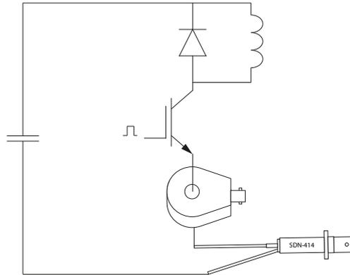
Figure 2.1 Measurement setup for testing Pearson 2878 and 50 mΩ shunt at low currents.
