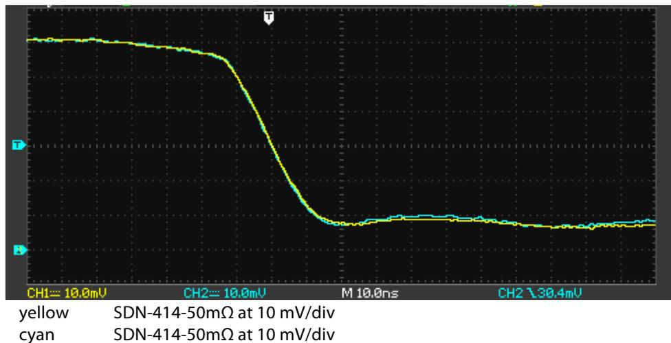
Figure 4.1.2 Identical response for same shunt connected with two BNC-cables to the oscilloscope.
