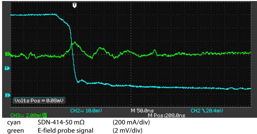
Figure 4.5.5 Responses of 50 mΩ shunt and response of E-probe near shunt leads.
