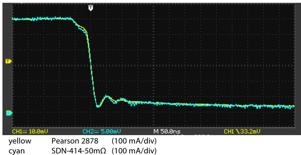
Figure 4.4.1 Responses for Pearson 2878 and shunt SDN-414-50 at 0.6 A.
